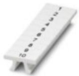
Zack marker strip, Strip, white, labeled, Printed vertically: consecutive numbers 1 ... 10, 11 ... 20, etc. up to 91 ... 100, mounting type: snap into tall marker groove, for terminal block width: 3.5 mm, lettering field size: 3.5 x 10.5 mm, Number of individual labels: 10
