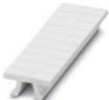
Zack marker strip, can be ordered: Strip, white, labeled according to customer specifications, mounting type: snap into tall marker groove, for terminal block width: 3.5 mm, lettering field size: 3.5 x 10.5 mm, Number of individual labels: 10
