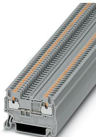
Feed-through terminal block, nom. voltage: 500 V, nominal current: 17.5 A, connection method: Push-in connection, 1 level, Rated cross section: 1.5 mm<sup>2</sup>, cross section: 0.14 mm<sup>2</sup> - 1.5 mm<sup>2</sup>, mounting type: NS 35/7,5, NS 35/15, color: gray
